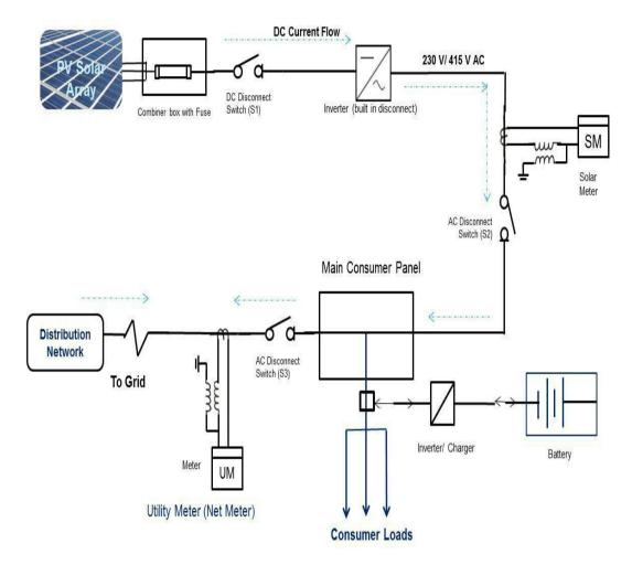
The utility meter (Net-meter) has to be bi-directional meter to register both import grid electricity amount as well as export solar electricity amount
